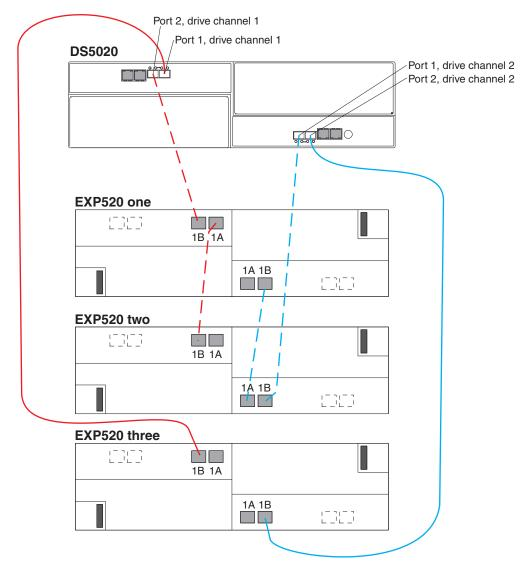
Figure 48. One DS5020 and three EXP520 storage expansion enclosures behind a pair of DS5020 drive ports
